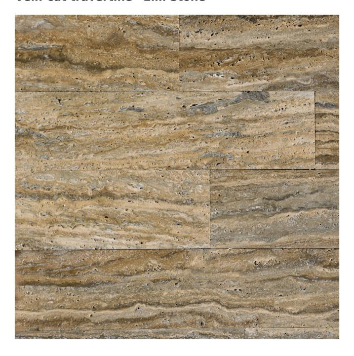
**Elm Stone** travertine comes from **material cut along the grain**, in which the typical intense structure of Rapolano Stone is very visible. This travertine has **marked veining ranging from grey to brown** against a beige background.
