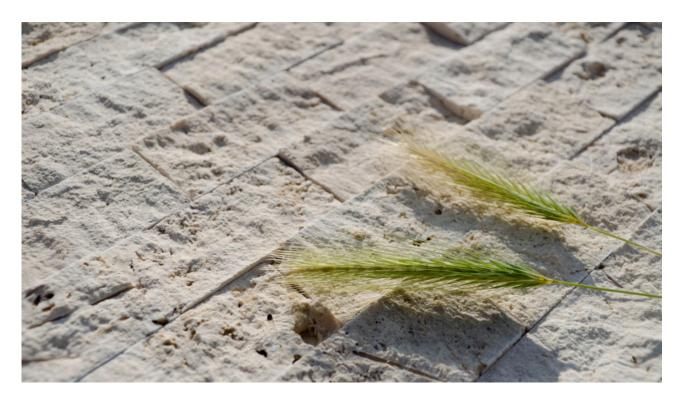
Wall mosaic in **classic travertine** with **natural split**. The rectangular strips,  $5 \times 10$  cm, are created by splitting the stone along the sedimentation line in order to obtain a variable surface.
